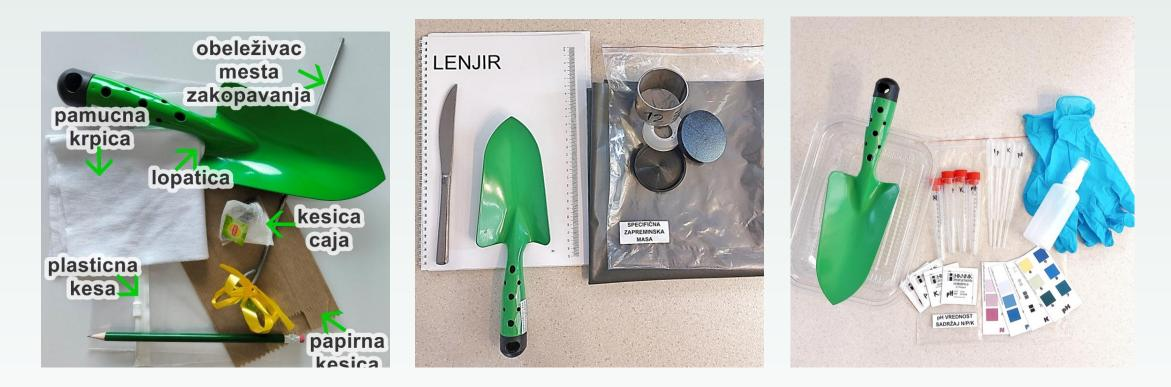
Materials for soil sampling and analysis were provided: tea bags, cotton cloth, shovel, reagents for chemical analyses, pipettes, test tubes, etc.
