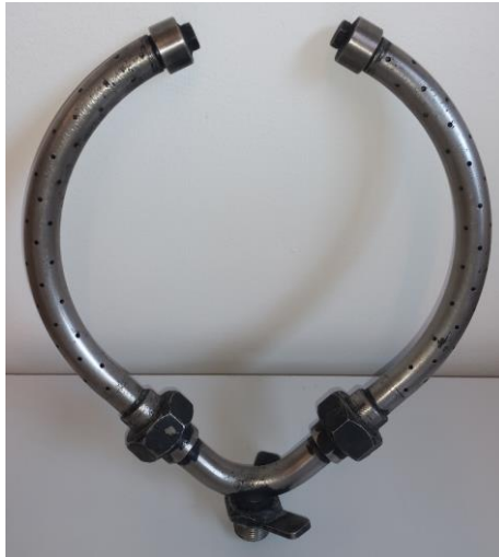
Fig. 1. Picture of the perforated annular nozzle that was used
