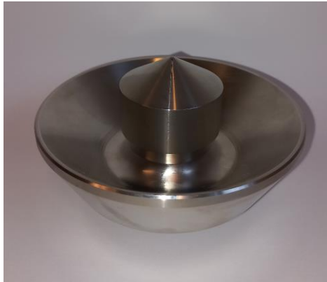
Fig. 4. Picture of the mushroom-cup nozzle that was used
