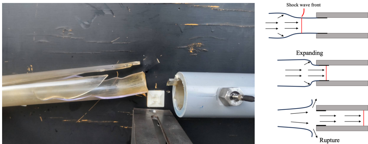
Fig. 9. Destruction part near sensor 1 at soft vinyl chloride 38/44mm (open)
