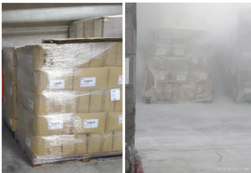
Fig. 2. The organic peroxides storage. Left photo showed the two pellets of C40-P on two weeks before the explosion. Right photo showed the fuming and partially melted PE films of the same pellet on 17:06 of the day of explosion. (Photos courtesy of Pingtung County Fire Department)
