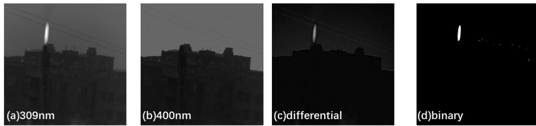
Figure 3. Results of photographing a hydrogen flame include (a) an image at 309 nm, (b) an image at 400 nm, (c) pixelwise differential of (a) and (b), and (d) the outcome of binary digitizing (c) with a threshold level of 75%
