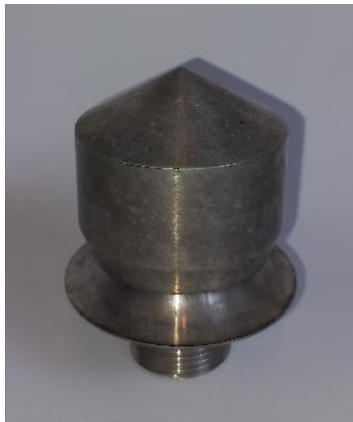
Fig. 6. Picture of the Janovsky-nozzle, taken from Janovsky et al. (2024)
