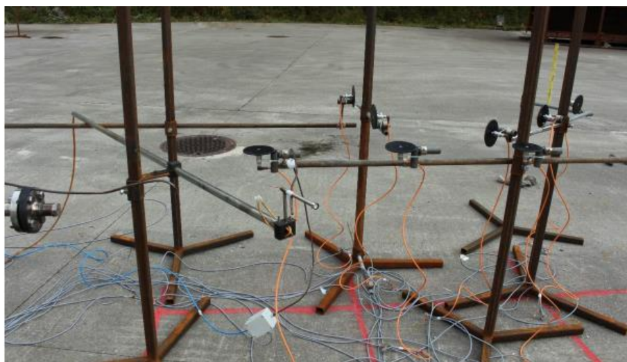
Fig. 3.: Photograph of the sensor layout and the orientation of the blast pressure plates
