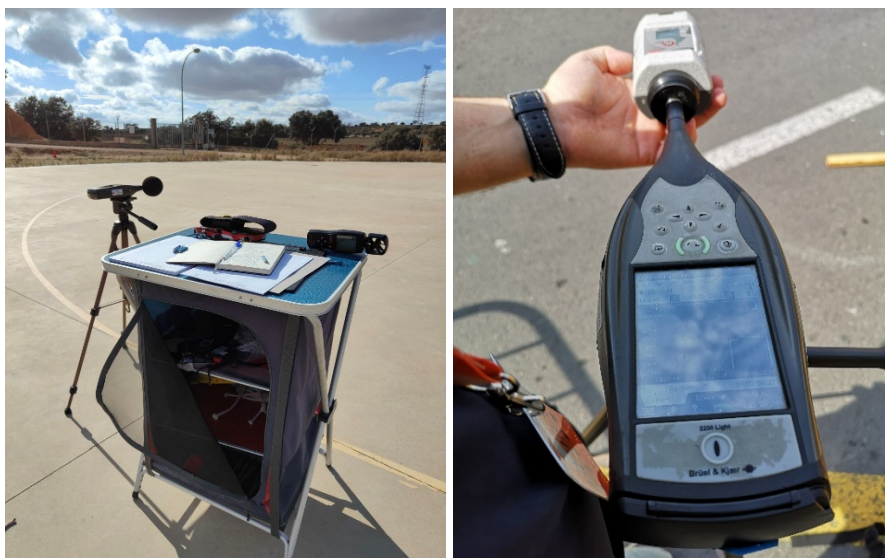
Fig. 1. Sound pressure level test setup.
