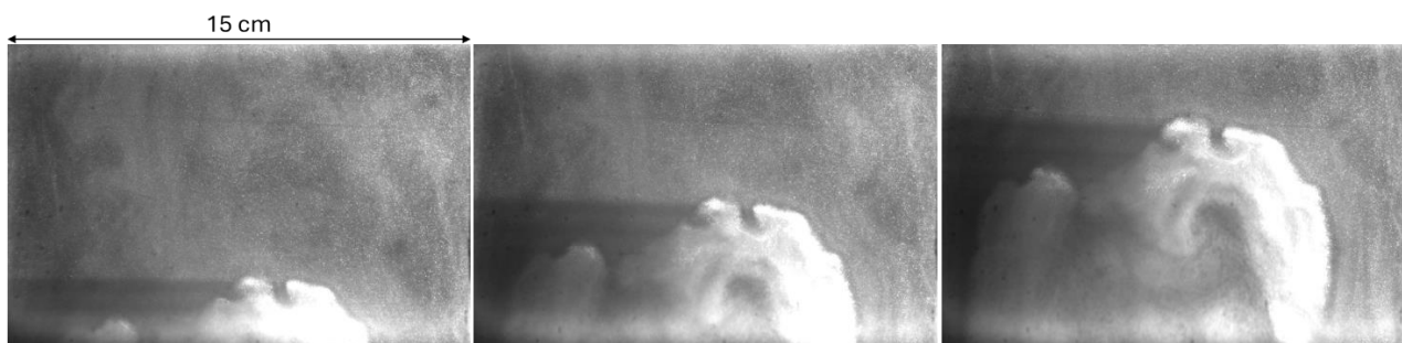
Fig. 2. Examples of raw TR-PIV images with the 20- \mu\text{m} powder (delay between images: 1 ms)
