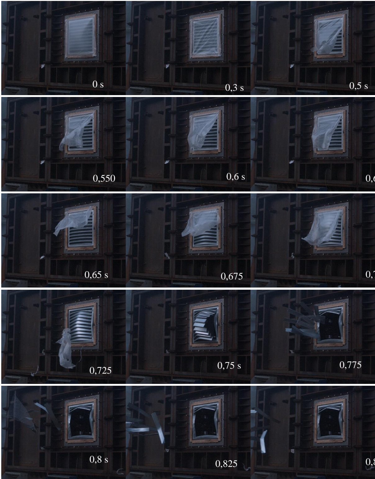
Fig 8. Sequence of images obtained by fast video of the grille opening for the 100 mbar test
