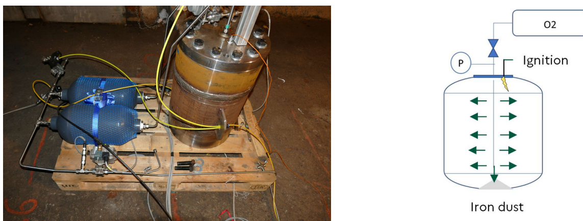
Fig. 1. View and scheme of the experimental setup of the explosion vessel
