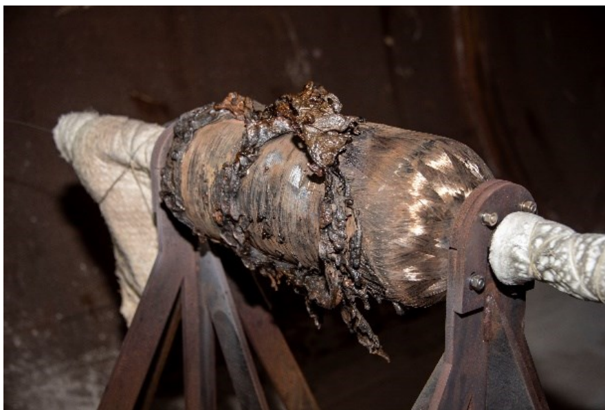
Fig. 9. Photo of the tank after the impinging hydrogen jet fire test
