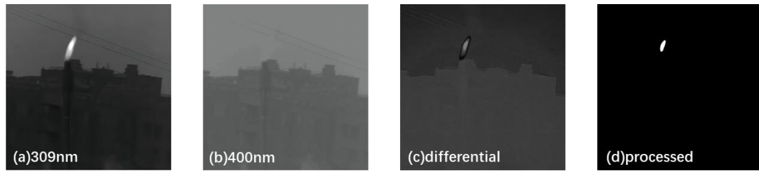
Figure 6. Experimental results of the simplified instrument: (a) image at 309 nm, (b) image at 400 nm, (c) pixelwise differential of (a) and (b), (d) processed image after applying Gaussian blur and binary digitization to
