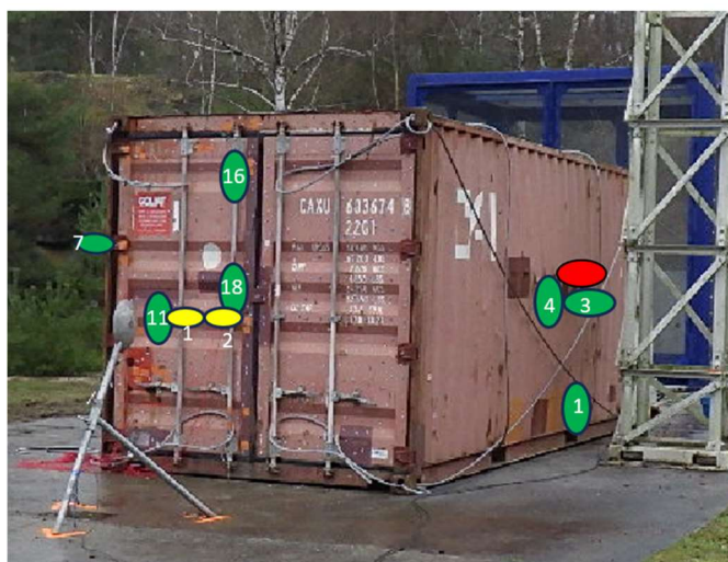
Fig. 4. Locations of some strain gauges (green), accelerometers (yellow) and the point aimed by the Laser (red) on the lateral wall and the door.
