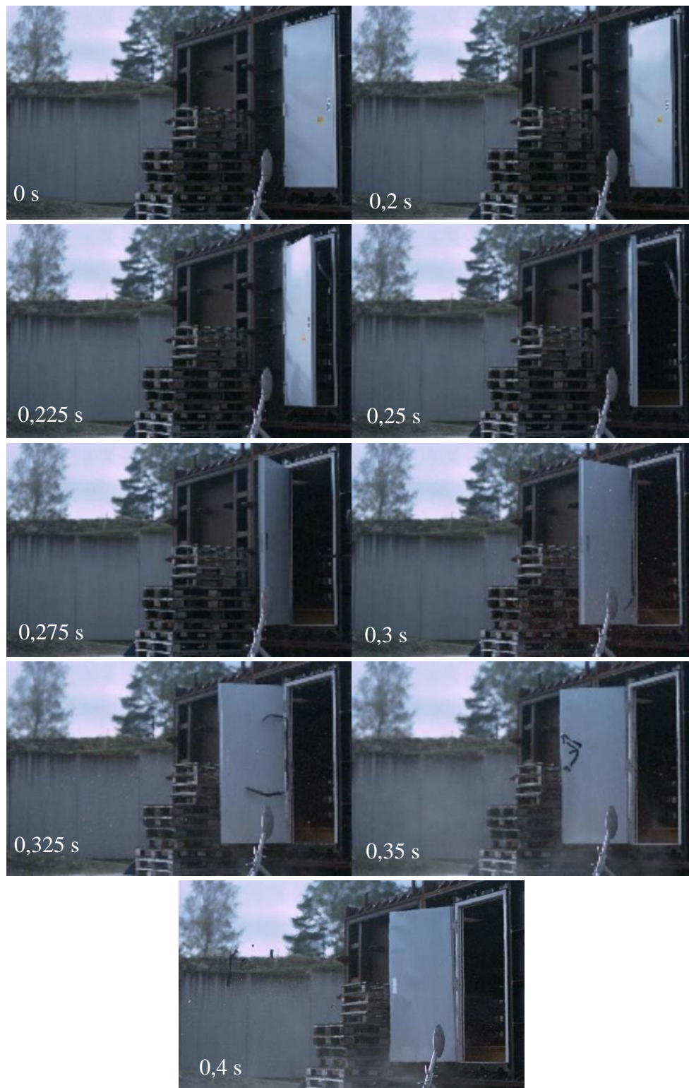
Fig 10. Illustration of door opening dynamics for 230 mbar overpressure
