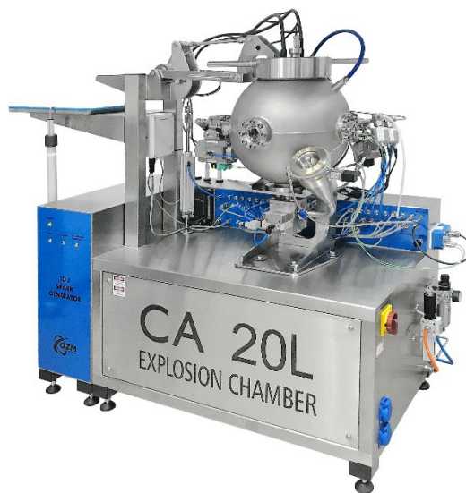
Fig. 1. The 20 dm 3 explosion chamber CA 20L by OZM Research.
