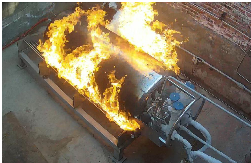
Fig.10. 500L liquid hydrogen storage tank fire test
