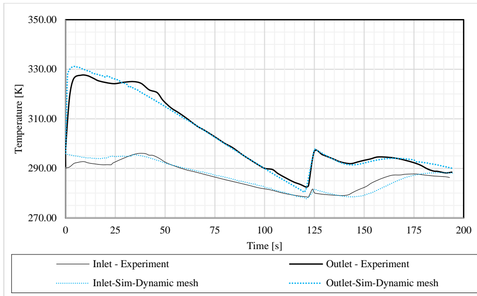
Fig. 6. Experimental and simulated temperature dynamics at the inlet (TE2) and outlet (TE3) of the PCV.
