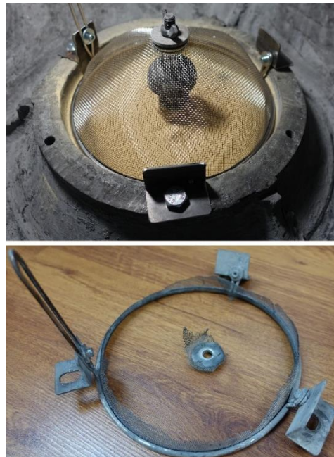
Fig. 10. Distribution system of the 365L-sphere before (with sieve) and after the explosion test (sieve completely burned) with aluminum
