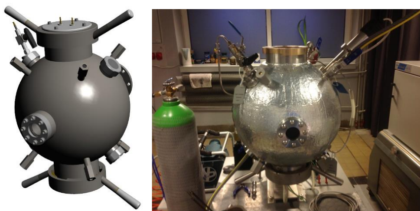
Fig. 1. 3D drawing (left) and the picture (right) of the 20 L combustion vessel.
