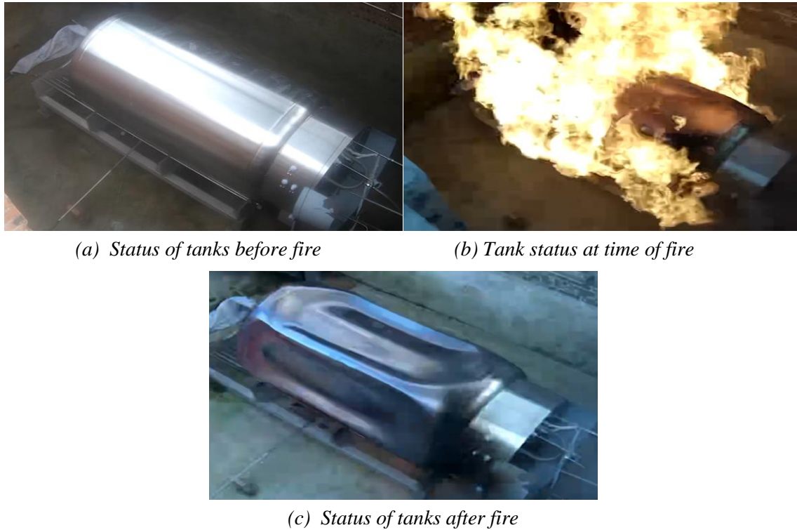
Fig.6. Changes in the state of storage tanks when subjected to fire
