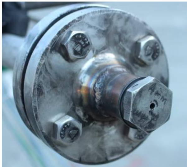
Fig. 2. Photograph of the 4mm-diameter nozzle used to mimic small puncture.
