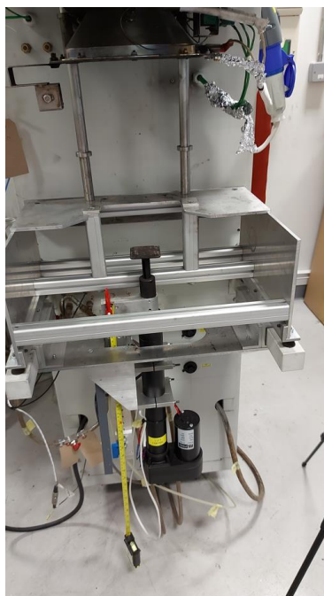
Fig. 4. Photo of the revised setup with the load cell element replaced with an actuator for the laboratory scale experiments
