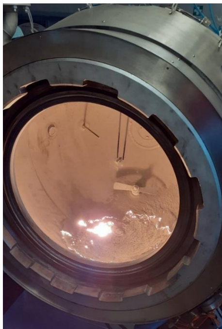
Fig. 9. 1m 3 after the explosion tests with aluminum. One can clearly see the still glowing aluminum on the bottom
