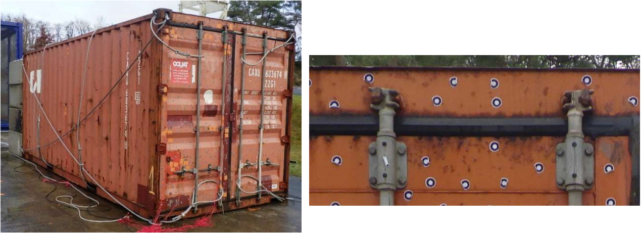
Fig. 1. Left: general view of the container N°1. Right: detailed view of the upper part of the closing system of the doors.
