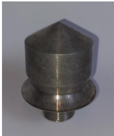
Fig. 5. Picture of the Janovsky nozzle that was used
