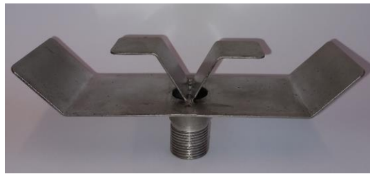
Fig. 2. Picture of the used rebound nozzle
