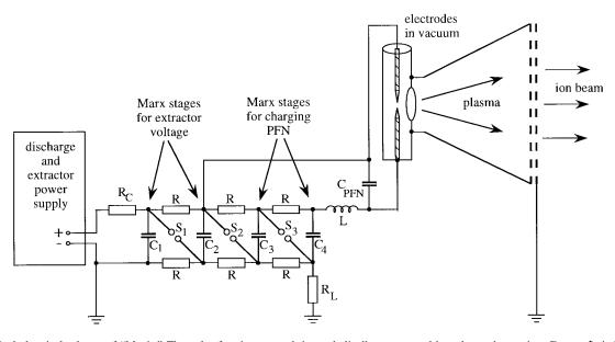
Fig. 2. Principal electrical scheme of "Magis." The pulse-forming network is symbolically represented by a lumped capacitor  $C_{\rm PFN}$ . L: inductive resistor (coil); the other notation is as in Fig. 1.
