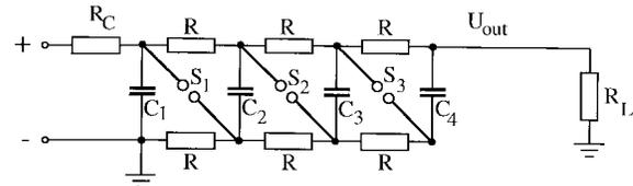
Fig. 1. Schematic of a four-stage Marx generator.  $R_C$ : charging resistor,  $R$ : stage-separating resistors,  $C_i$ : capacitors,  $S_i$ : switches (spark gaps),  $U_{out}$ : output voltage;  $R_L$ : load.
