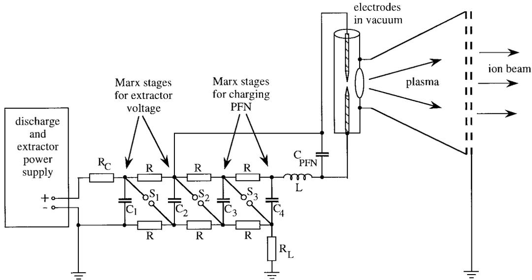
Fig. 2. Principal electrical scheme of “Magis.” The pulse-forming network is symbolically represented by a lumped capacitor  $C_{\text{PFN}}$ .  $L$ : inductive resistor (coil); the other notation is as in Fig. 1.
