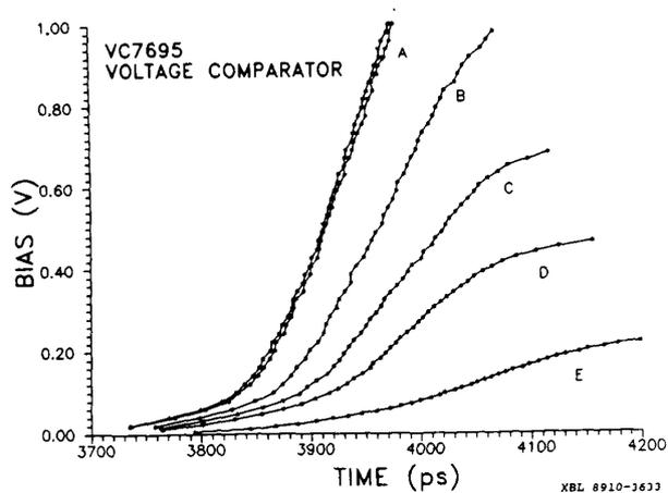
Fig. 6. VC7695 comparator response to 120 ps rise time pulses of amplitudes (a) 1.31V, (b) 0.98V, (c) 0.69V, (d) 0.48V and (e) 0.245V.
