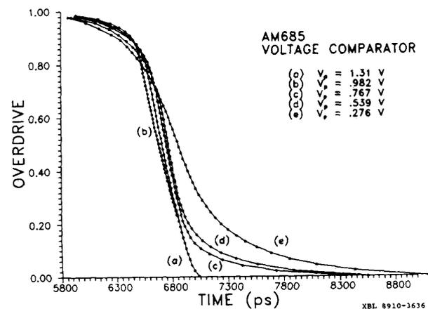
Fig. 9. Normalized time walk of AM685 comparator.
