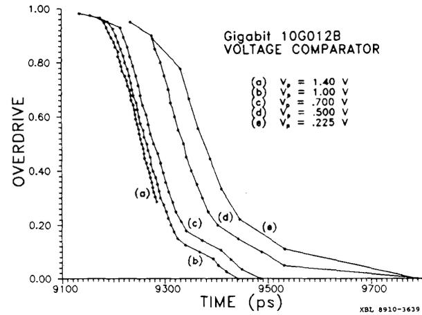
Fig. 12. Normalized time walk for 10G012B GaAs comparator.
