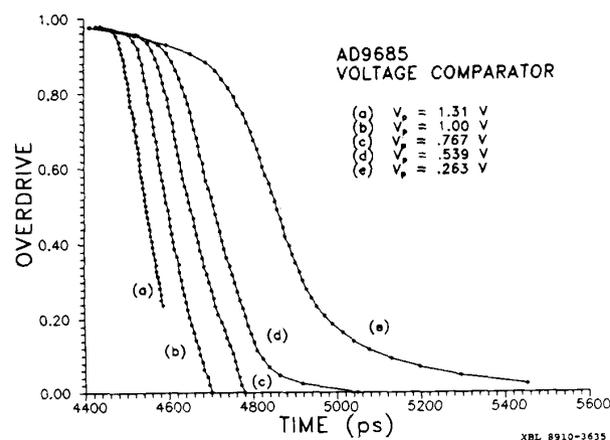
Fig. 8. Normalized time walk of AD9685 comparator.
