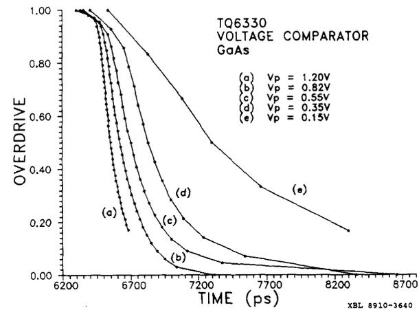
Fig. 13. Normalized time walk for TQ6330 GaAs comparator.
