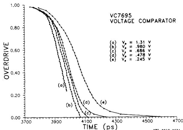
Fig. 7. Normalized data from Fig. 6 showing comparator time walk as function of overdrive ratio  $r_i = (V_i - V_{thr}) / V_i$ .
