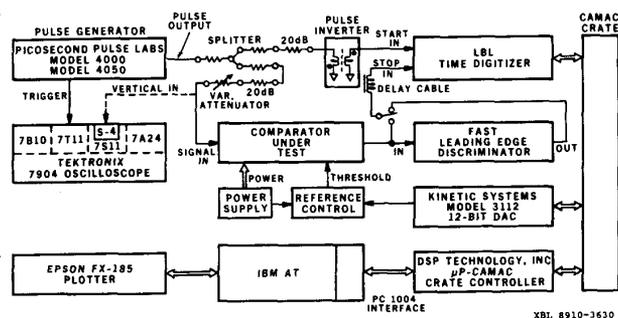
Fig. 3. Block diagram of the measurement system.
