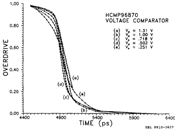
Fig. 10. Normalized time walk of HCMP96870 comparator.
