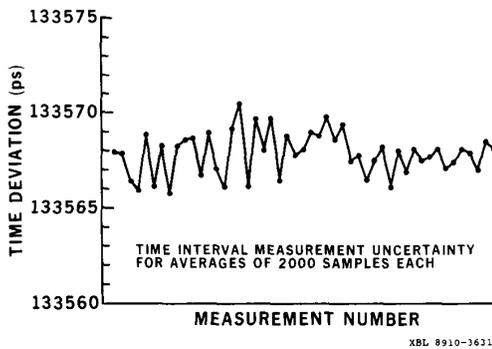
Fig. 4. Statistical timing error of the system in Fig. 3. Fixed time interval of 133.565 ns was measured 40 times with 2000 samples each.
