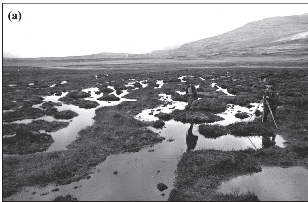
Figure 5(a) Theodolite being levelled at a survey point; (b) Sampling of a peat core at a survey point using a ‘Russian Sampler’
