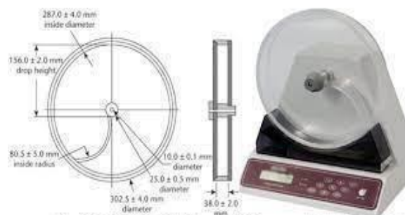
Fig: Roche Friabilator For Uncoated Tablets
