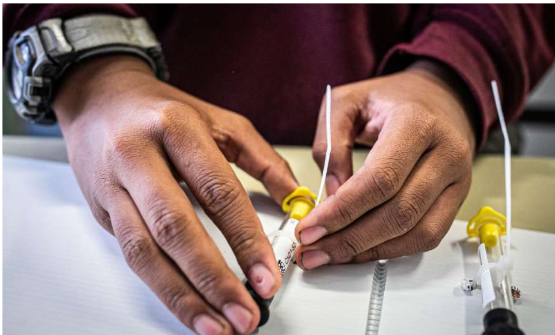
Image 21 CurieuzeNeuzen - The measuring tubes are attached to a measuring board. These tubes collect NO 2 , an indicator for traffic. Credit: Bas Bogaerts (BE), CC BY-SA 4.0
