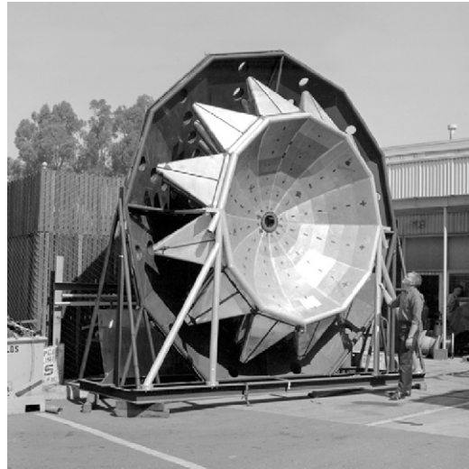
Fig. 5. The “Dish”—A scintillation counter array used to study the \pi-\pi interaction.
