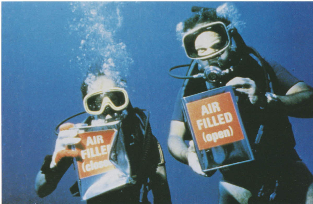
Fig. 2. Boyles law in action: the mechanism of barotrauma. The can on the right was open on the bottom to allow water to enter and equalize the pressure in the gas space on descent. The can on the left was closed and pressure equalization was achieved by collapse of the can. (Photograph courtesy of Dr. Richard Vann)
