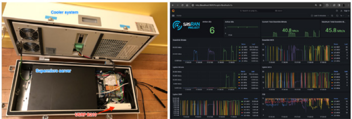
Figure 3 Inside of the supermicro server (left) and GUI of the 5G testbed (right)
