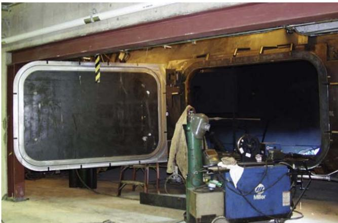
**Fig. 9.** Large target access door.
