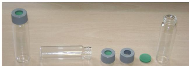
**Fig. 1.** Typical volatile organic compound (VOC) sampling vials with caps which allow for a gas sample to be withdrawn from the headspace of the vial without removing the cap. These vials should be filled approximately  $\frac{3}{4}$  full with soil, mud, water, vegetation, etc.
