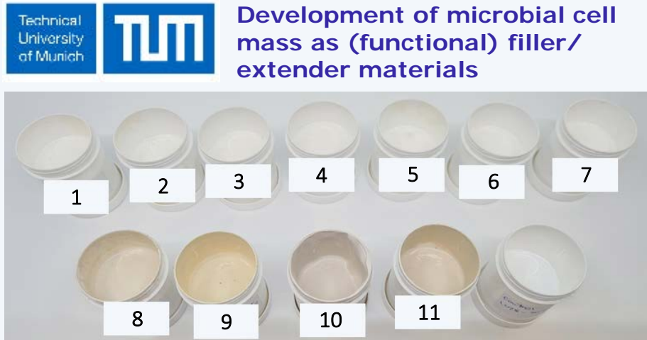
PVC 80 formulations containing bio-based fillers (1-11), calcium carbonate control. Chemically modification (1-7) for improved color properties
