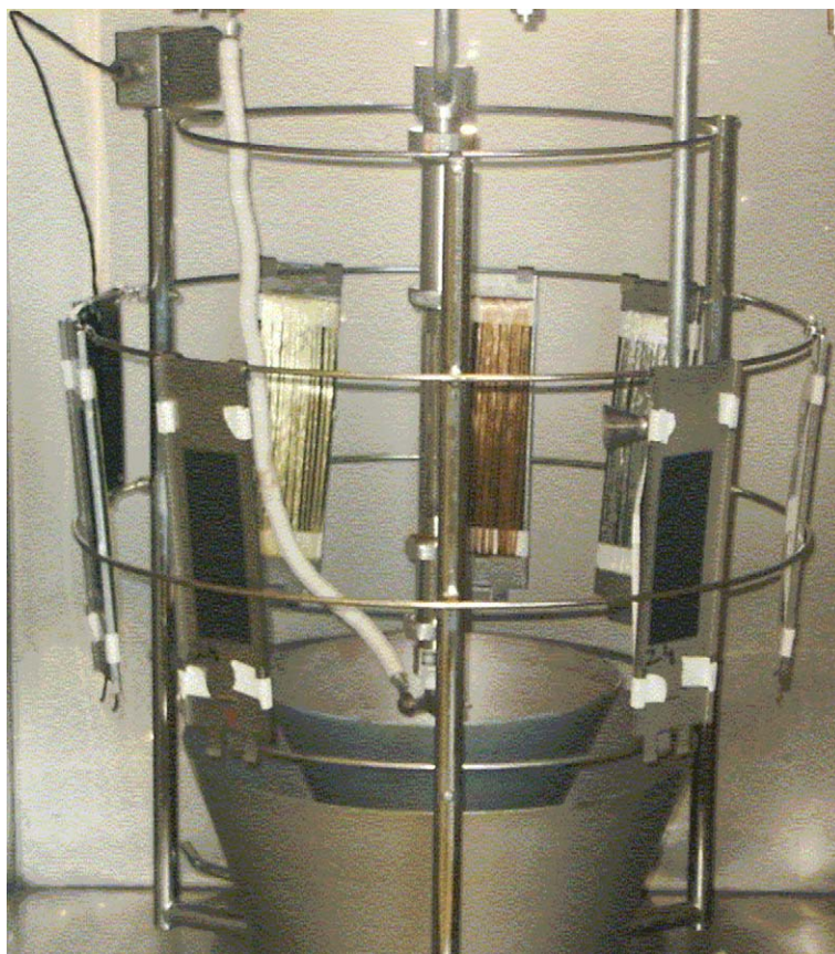
Fig. 1. Rack of the Atlas 3 Sun Weatherometer with samples loaded and ready for exposure to UV radiation.
