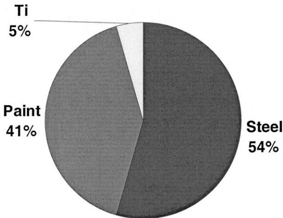
Fig. 5. Composition of orbital debris causing 22 perforations of the radiator facesheet over 50 missions from STS-50 to STS-110.
