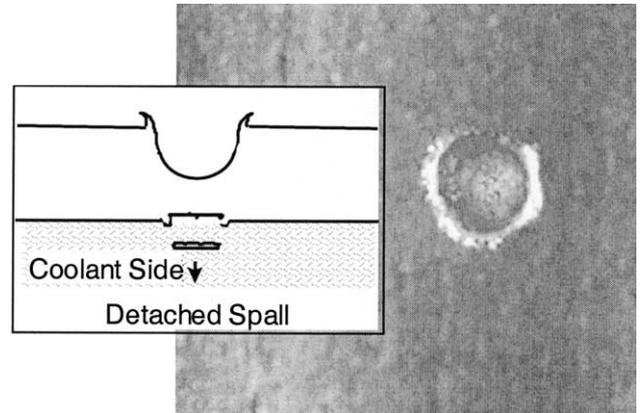
Fig. 6. Deep crater (0.8-mm diameter by 0.47 mm ) in 0.9-mm thick aluminum interconnect line. Inset illustrates how detached spall occurred from under the crater. SEM/EDX indicated a steel debris impactor.
