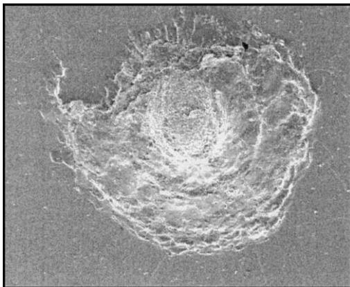
Fig. 2. STS-92 left-hand #2 window crater (10-mm diameter by 1.9-mm deep) caused by orbital debris (paint).
