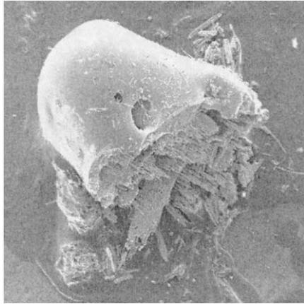
Fig. 7. SEM image of 1.5 mm × 1 mm × 1 mm lead/tin particle extracted from STS-73 FRSI impact crater. From its morphology and structure, this grain appears to be a piece of solder with small amounts of electric circuit board attached at an end. The fibers in the circuit board contain silicon and calcium with minor aluminum present.
