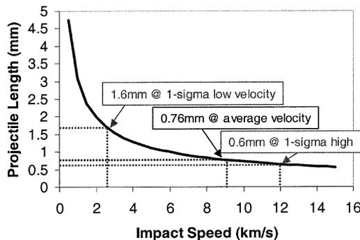
Fig. 8. Particle size sensitivity analysis considering 1σ variation in possible debris impact velocities for the STS-92 window #2 impact shown in Fig. 3.
