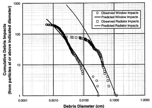
Fig. 9. Comparison of actual window (in squares) and radiator (in circles) damage to predicted (lines) cumulative for 28 flights: STS-50, 56, 71, 72, 73, 75, 76, 77, 79, 80, 81, 84, 85, 86, 87, 88, 89, 91, 94, 95, 96, 106, 92, 97, 98, 104, 108, and 109.
