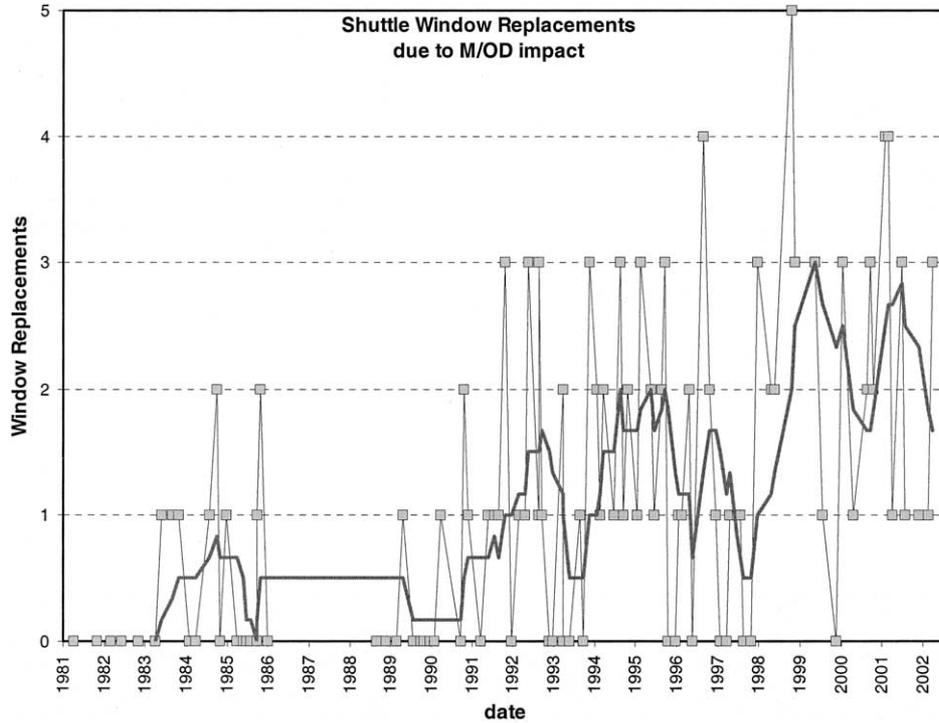
Fig. 4. Window replacements from M/OD impact with the bold line indicating the trend over a 6-mission running average.
