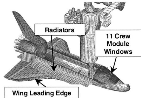
Fig. 1. Orbiter surfaces inspected for M/OD impact damage.
