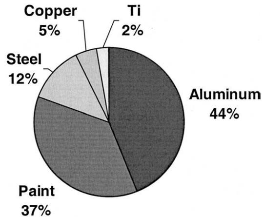
Fig. 3. Composition of orbital debris particles that caused 41 window replacements during the period from STS-50 (June 1992) to STS-110 (April 2002).
