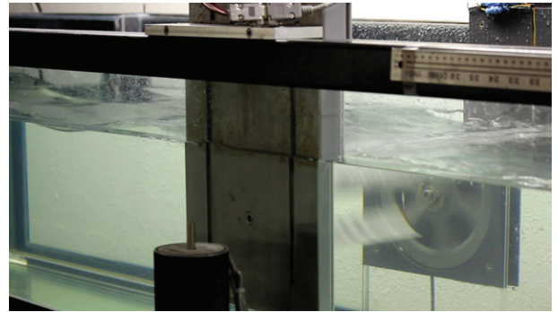
Fig. 10. Picture of wave cancellation from downwave above. For experimental parameters see caption of Fig. 9.
