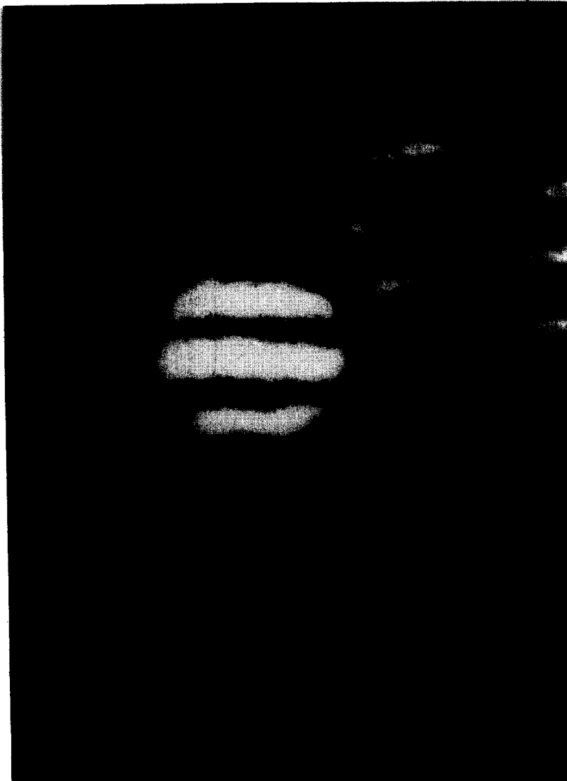
Fig. 16. Twyman-Green interferogram of the Er:YALO laser rod used in this work. For this measurement both faces of the laser rod had broadband AR coatings.
