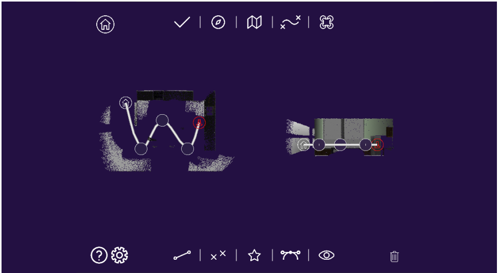
Figure 29. Adding the last key point (the landing point) to the environment map
