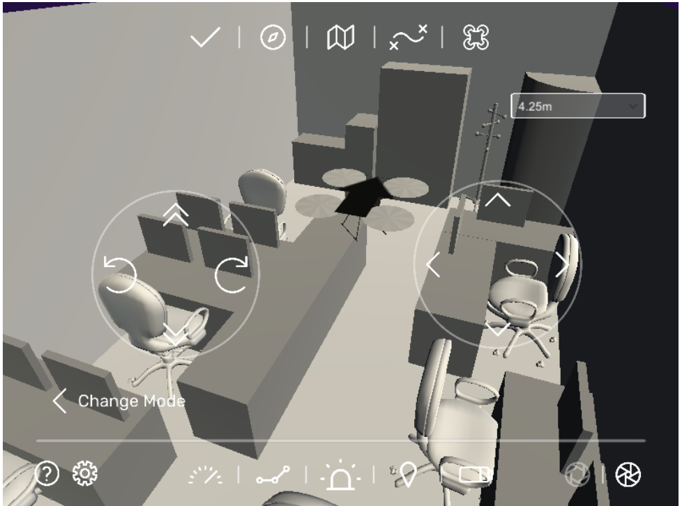
Figure 18. Sequence of a typical scanning session; the walls and environment appear on the screen as the drone moves around
