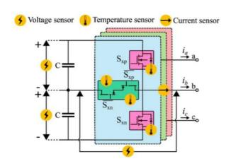
Image 3: Scheme of a low-power converter module with its respective sensors
