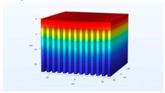
Image 1: The results of temperature distribution in the designed air cooled heatsink
