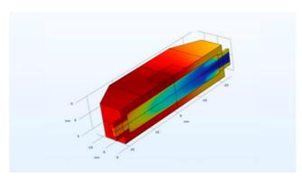
Image 2: The result of temperature distribution in the liquidcooled heatsink
