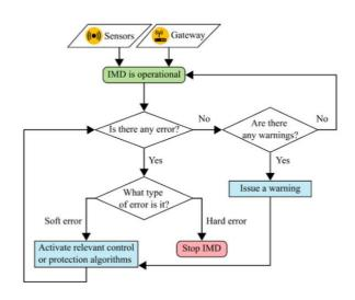
Image 4: Flowchart of the proposed fault tolerance algorithm
