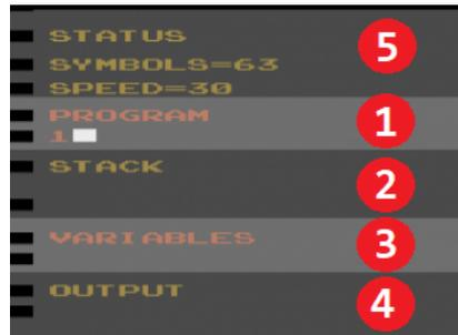
Figure 2: Main display of Atari 2600 BASIC programming with the editor (1), stack (2), variable values (3), output (4), and status (5). The region that shows the graphics are not visible in this Figure.
