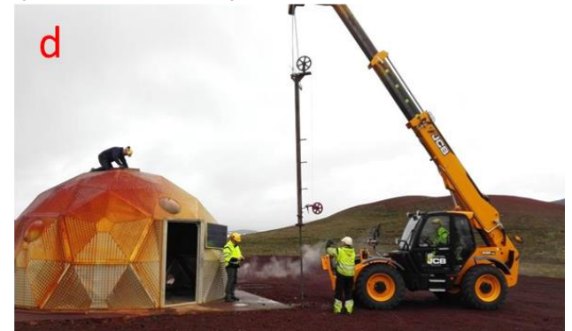
Figure 20: Pictures of the experiment accomplished at KJ-35 well (Krafla, Iceland). a) Tube containing micro-reactors is inserted in a bigger tube; b) the device is hosted over the well and it will be lowered through a pulley controlled by a motor hosted in a ÍSOR van; c) recover of the of the device through the pulley controlled motor; d) final recover of the tube containing the micro-reactors.
