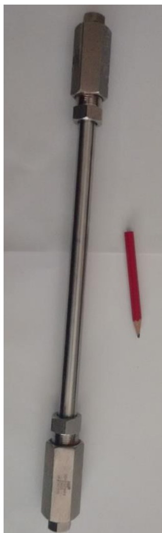
Figure 11: Picture of micro-reactor, model MS-15 HiP (from the High Pressure Equipment Company).
