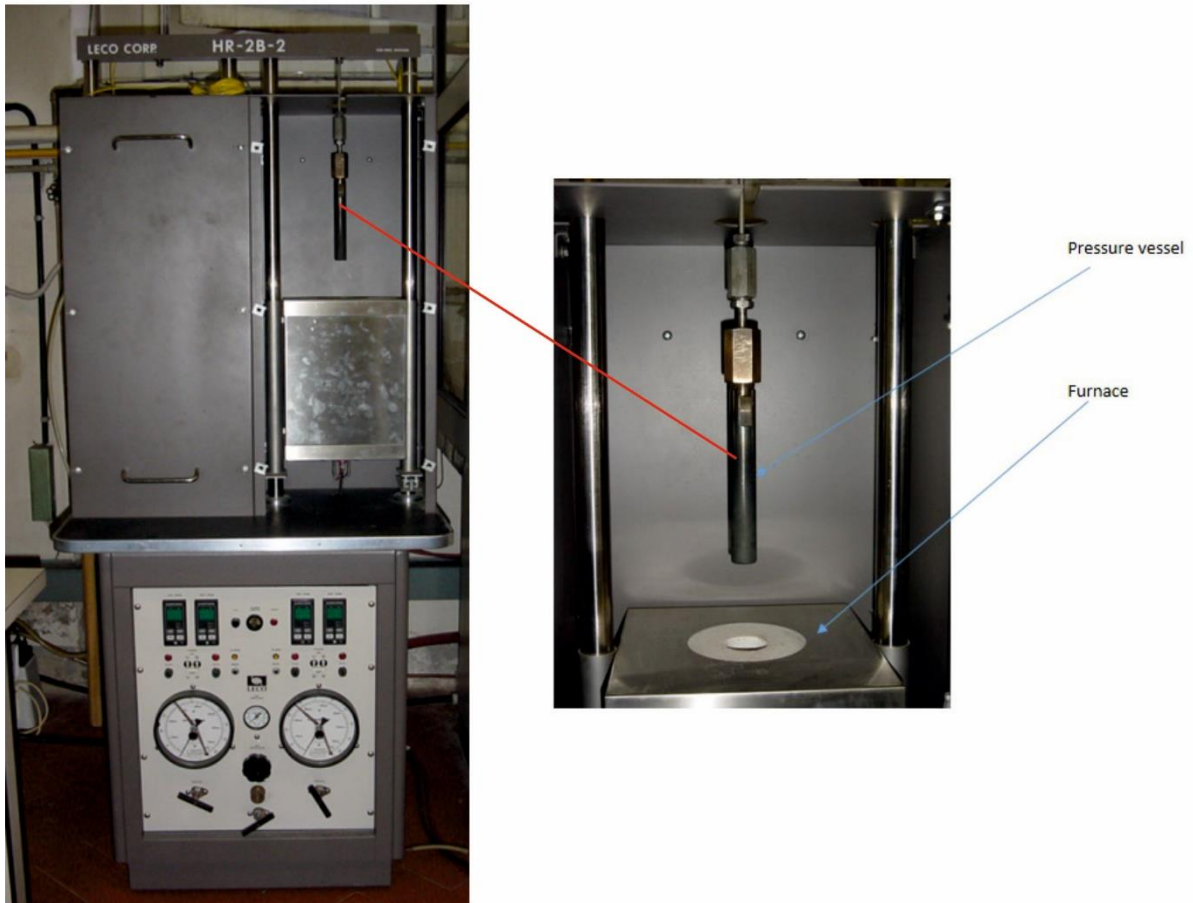
Figure 4: The HR-2B-2 cold seal pressure vessel (left) and a detail showing the René 41 pressure vessel containing Au capsule(s) approaching to enter into a sliding furnace (right).
