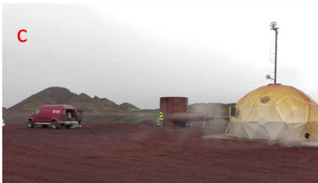
Figure 20: Pictures of the experiment accomplished at KJ-35 well (Krafla, Iceland). a) Tube containing micro-reactors is inserted in a bigger tube; b) the device is hosted over the well and it will be lowered through a pulley controlled by a motor hosted in a ÍSOR van; c) recover of the of the device through the pulley controlled motor; d) final recover of the tube containing the micro-reactors.
