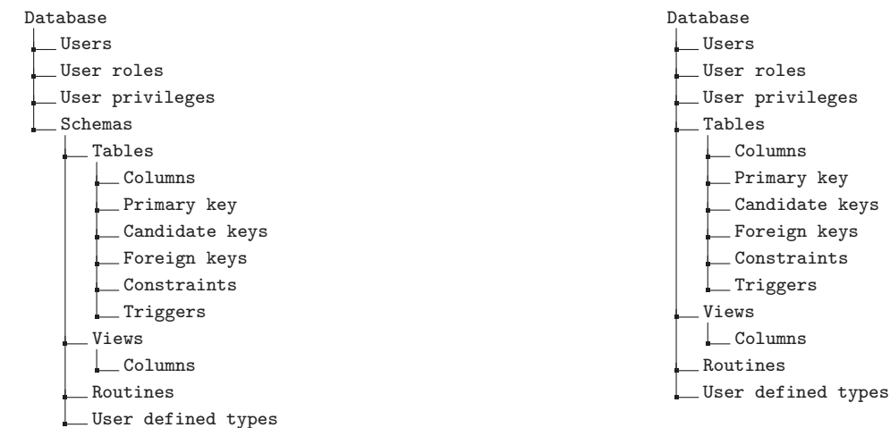
Figure 4: Database structure as an hierarchy.
