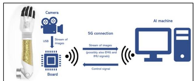
Fig. 8. Architecture of the application for the Adaptive Control of Hannes Prosthetic Device use case
