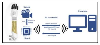
Fig. 8. Architecture of the application for the Adaptive Control of Hannes Prosthetic Device use case
