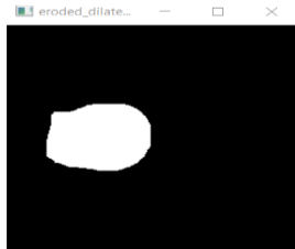
Figure 7: After Erosion & Dilation Image
