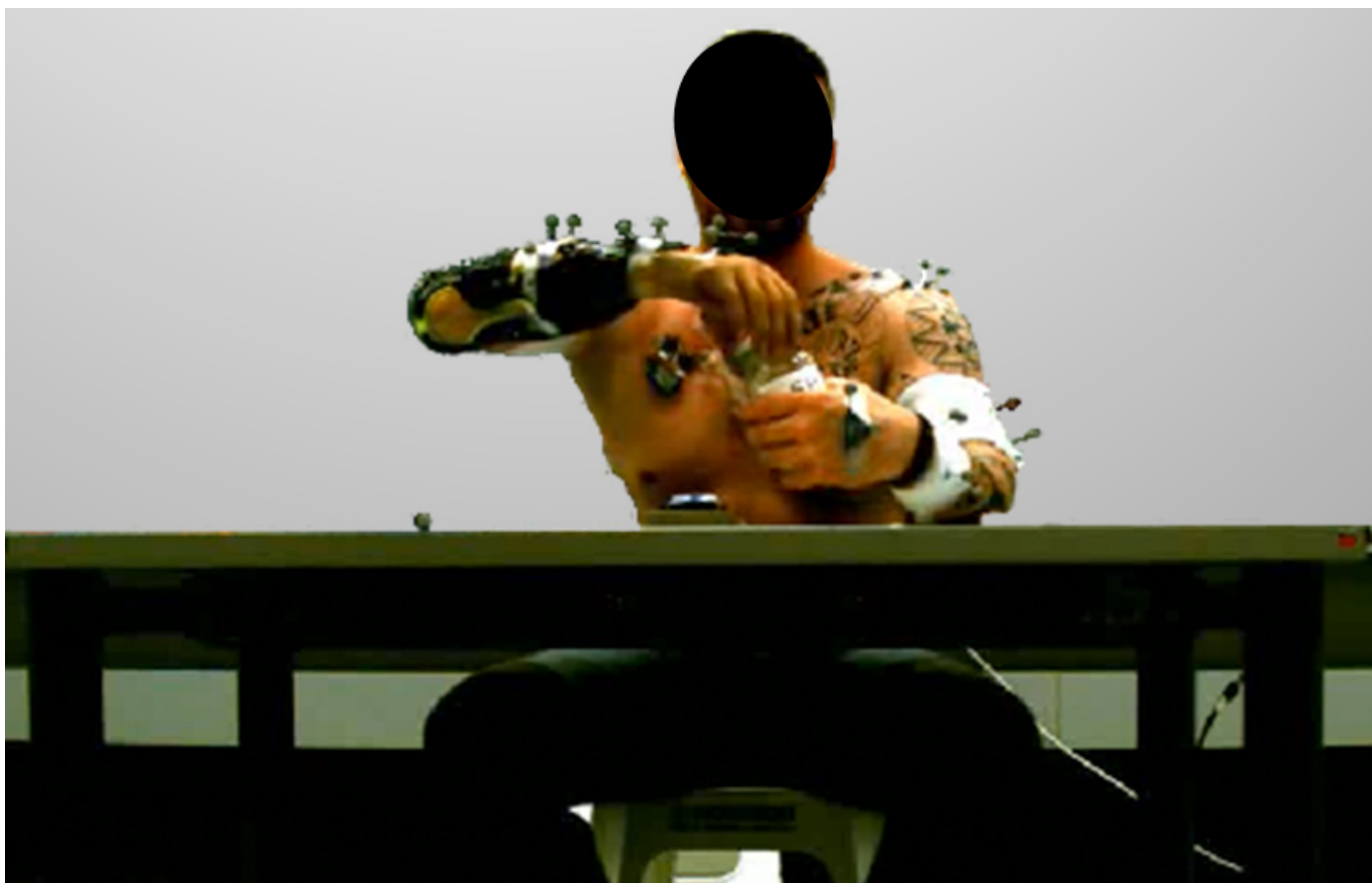
Figure 1: Prosthesis user equipped with Michelangelo Hand (Otto Bock Healthcare GmbH) and two electrode conventional control performing the SHAP - Test task „jar lid“. 63 retroreflective markers and 14 EMG channels were attached to the trunk and upper extremities.
