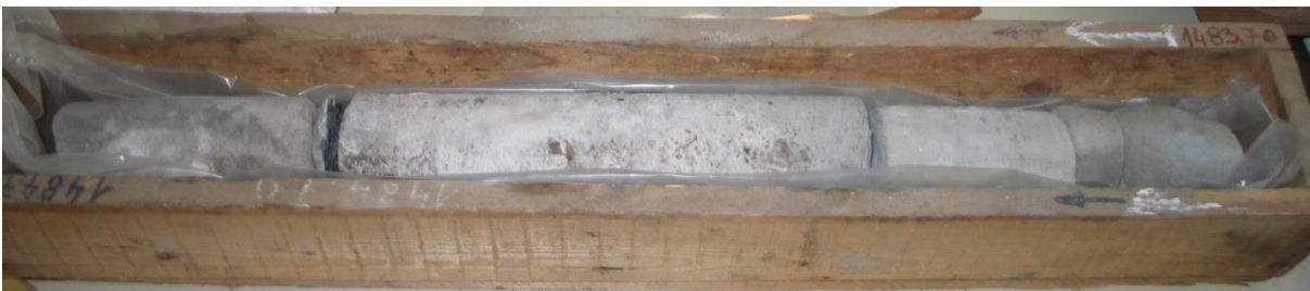
Figure 35 Core of the Upper Miocene loose sandstone formation into which reinjection of water has to be established
