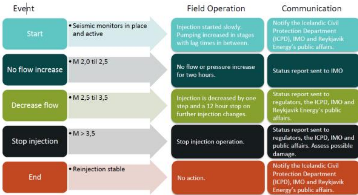
Figure 16 Reykjavik Energy's work procedure for large scale reinjection after a temporary shutdown or when significant changes are made in reinjection from the power plant. The procedure is modeled after AltaRock Energy's decision tree for triggers and mitigation actions from its Newberry EGS demonstration project Reykjavik Energy's work procedure for large scale reinjection after a temporary shutdown or when significant
