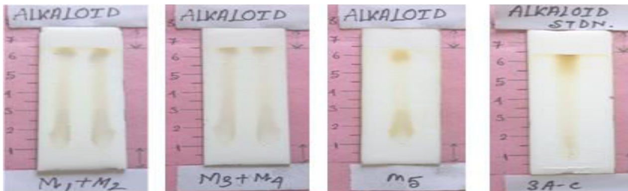
Figure.18 Alkaloid TLC profile by doubling each ingredient
