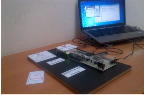
Figure 7. The RFID top up circuit
