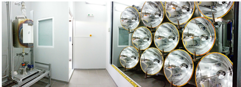
Fig. 17. High-flux solar simulator and reactor integrated set-up.
