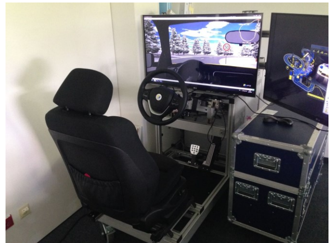
Fig. 5. The static System Experience Platform driving simulator.
