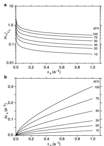
Fig. 5. Plots of the fractional increase in longitudinal strain rates (a), and the strain-rate increase (b), against the preperturbation strain rate, for various values of the perturbation in longitudinal stresses ( $\Delta F/S$  in kPa).
