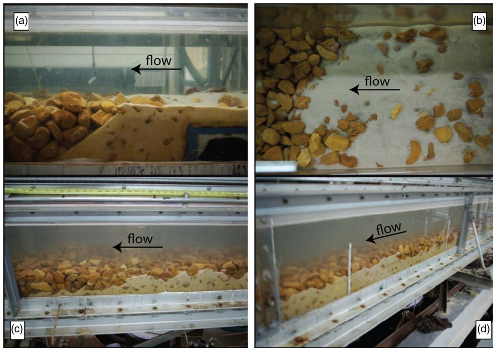
Fig. 3. Photographs of sand fill process: (a) side view of filling bed at low discharge; (b) top view of filling at low discharge; (c) side view of filling at high discharge; (d) side view of filling at high discharge at a later time
