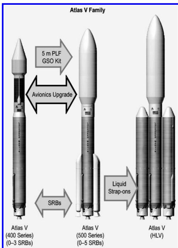
**Fig. 9** Atlas V family of launch vehicles.**Table 10 RD-180 engine characteristics**
