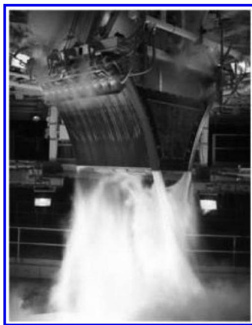
Fig. 12 XRS-2200 aerospike engine.
