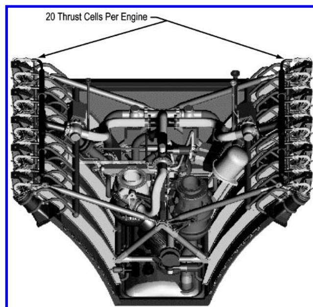
Fig. 11 X-33 aerospike engine.
