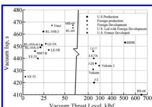
Fig. 3 Existing LO<sub>2</sub>/LH<sub>2</sub> engine production level designs.
