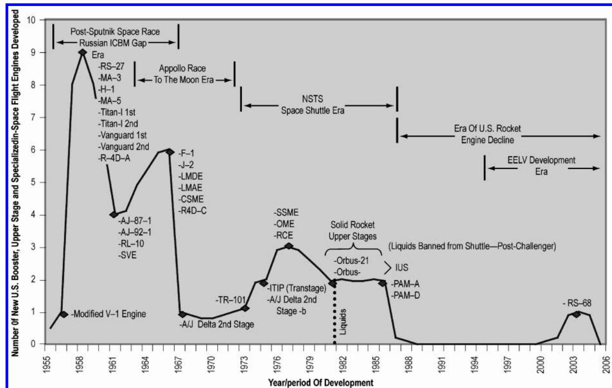
Fig. 2 U.S. rocket engine developments from 1955–2005.
