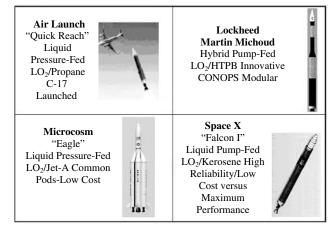
Fig. 10 Vehicle characteristics for the four contractors in phase IIa for the DARPA FALCON program [2].
