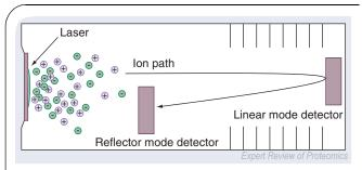
Figure 1. Schematic of laser desorption/ionization time-of-flight mass spectrometry. Laser excitation of samples (or sample-matrix mixture in the case of matrix-assisted laser desorption/ionization) results in desorption of ionized species that then drift into the time-of-flight tube and are detected in either linear or reflector mode.
