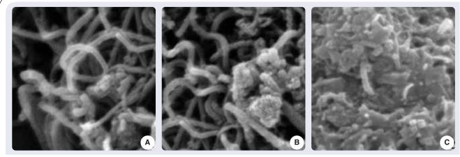
Figure 2. Scanning electron microscopy images of (A) multiwalled carbon nanotube layer, (B) a nanotube layer in the presence of an immobilizing polymer and (C) a nanotube layer immobilized in a polymer after sample spotting. Reprinted with permission from [18] © 2005, Elsevier, The Netherlands.
