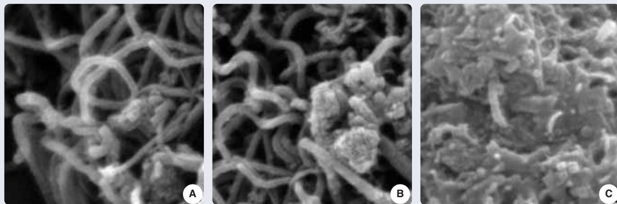
**Figure 2.** Scanning electron microscopy images of (A) multiwalled carbon nanotube layer, (B) a nanotube layer in the presence of an immobilizing polymer and (C) a nanotube layer immobilized in a polymer after sample spotting. Reprinted with permission from [18] © 2005, Elsevier, The Netherlands.
