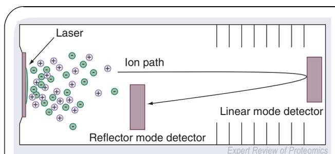
**Figure 1. Schematic of laser desorption/ionization time-of-flight mass spectrometry.** Laser excitation of samples (or sample–matrix mixture in the case of matrix-assisted laser desorption/ionization) results in desorption of ionized species that then drift into the time-of-flight tube and are detected in either linear or reflector mode.
