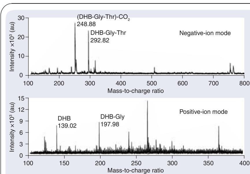
Figure 3. Surface-assisted laser desorption/ionization mass spectrometry of bacillibactin hydrolysate on nanoporous silica films. Subunits of bacillibactin were identified by analyzing the hydrolysate in positive- and negative-ion mode, firmly establishing the components of this siderophore. au: Arbitrary units; DHB: 2,5-dihydroxybenzoic acid.
