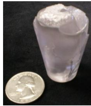
Figure 7: (a) Furnace used at Crystal Systems to grow sapphire by the Heat Exchanger Method. (b) The first sapphire boule grown at Watertown in 1967. (c) Production-quality 34-cm-diameter sapphire boule. Courtesy Crystal Systems, Inc.
