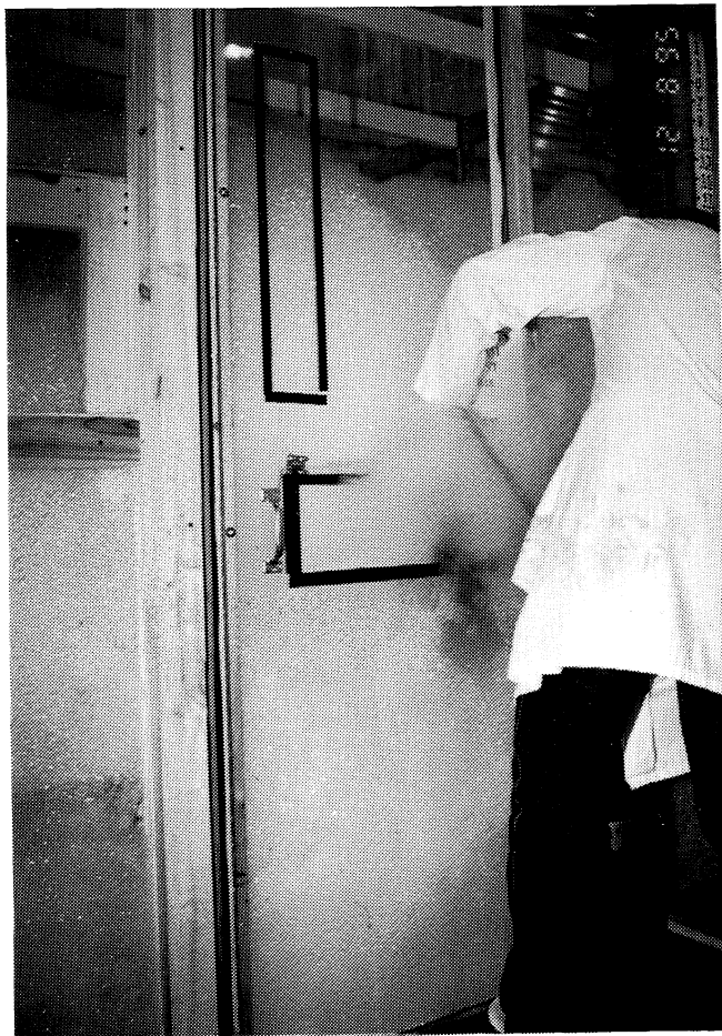
Figure 4. CO 2 Fire Extinguisher Foam Knockdown Through Foodslot
