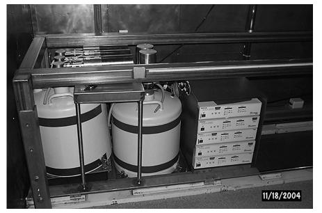
Figure 1. Coaxial germanium measurement system.
