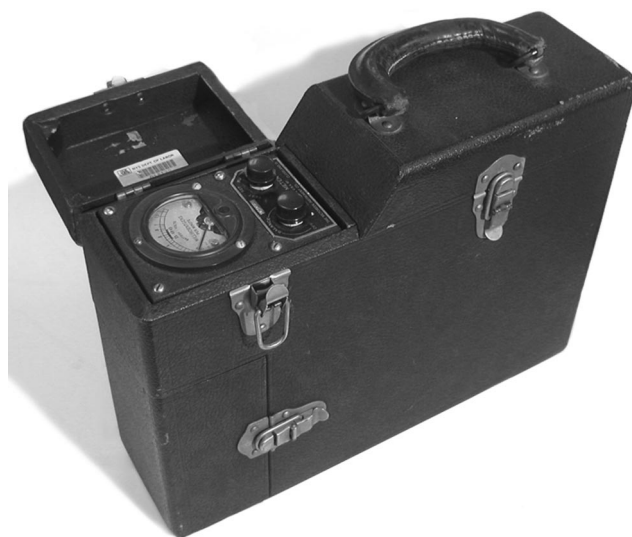
Fig. 8. Ion chamber manufactured by Victoreen (ca. 1945). This model seems to have been the first commercially available survey meter. The cylindrical chamber is located behind the latched door on the front end of the case.
