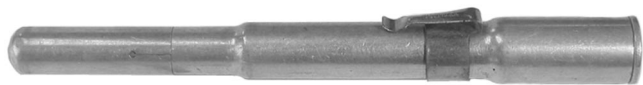
Fig. 6. Pocket dosimeter built by Charlie Lauritsen and given to Robley Evans (1932). The unitless scale reads 0–50. Almost certainly the world’s oldest pocket dosimeter.
