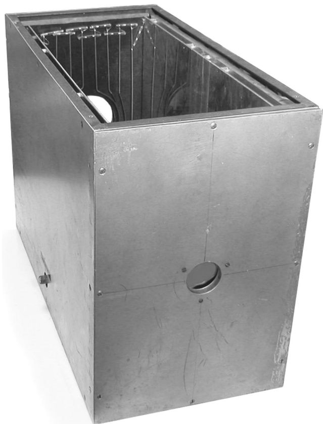
Fig. 4. Herb Parker's free-air ionization chamber (1935–1940). The top cover has been removed so that the guard wires on the back wall of the chamber can be seen.
