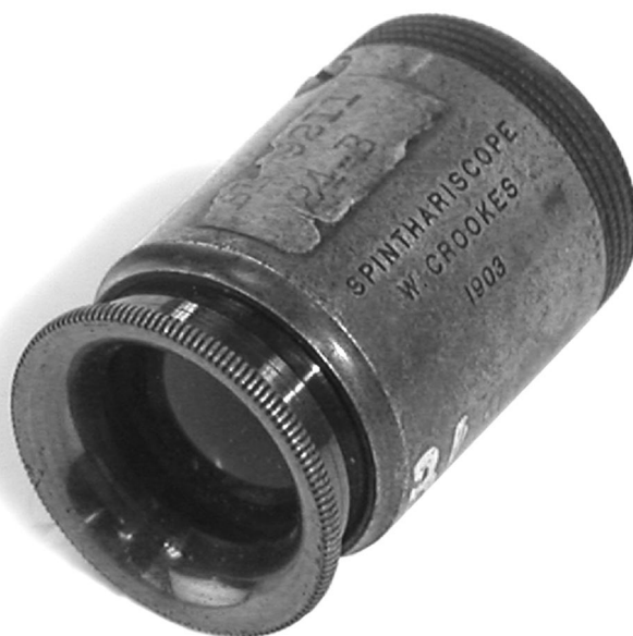
Fig. 16. Crookes spintharoscope from Robert Millikan's laboratory (ca. 1910–1920). This version of the spintharoscope would have been used for demonstration purposes, not quantitative measurements.
