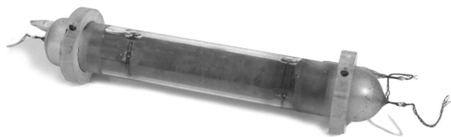
Fig. 10. Hand-built GM tube (1940's). The wall of the tube is glass and a cylindrical copper tube serves as the cathode. Note that the ends of the tube have been coated with wax to reduce leakage currents.
