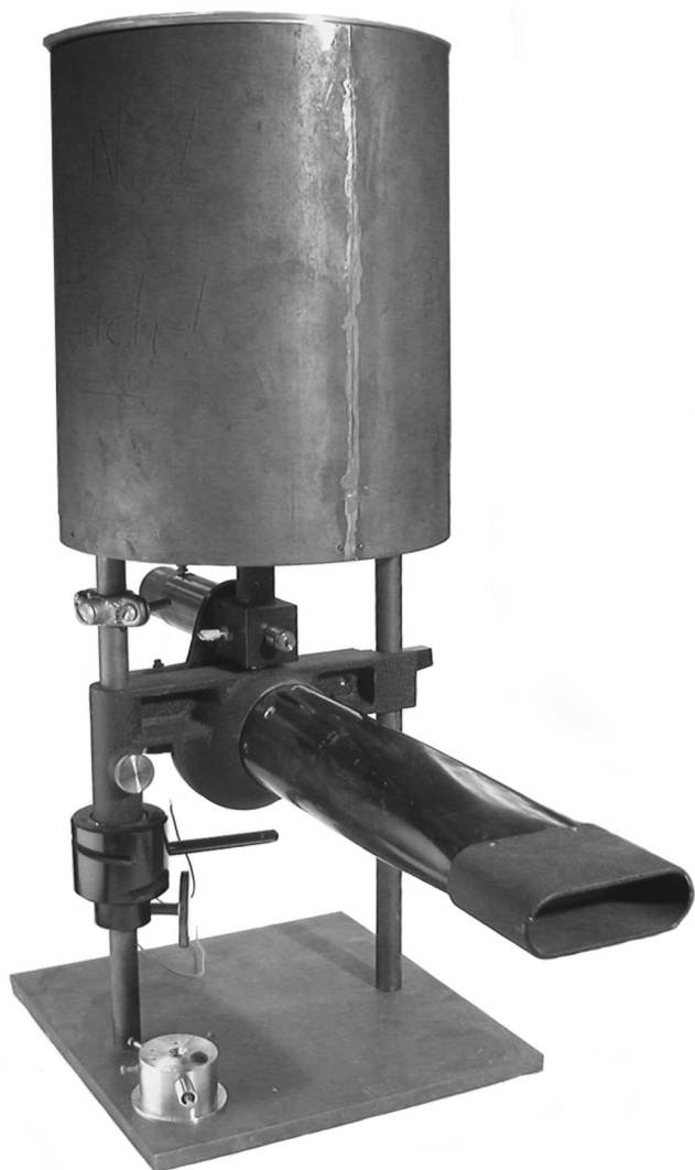
Fig. 7. Four pi ionization chamber built and used at the National Bureau of Standards (ca. 1953). The collected charge from the chamber is determined with a Lindemann-type electrometer that has been removed from the unit and placed on the lower left corner of the base for visibility.
