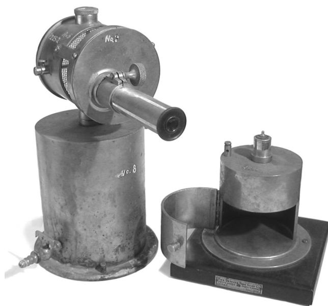
Fig. 5. Lind electroscope (ca. 1920–1930) with two interchangeable chambers. The electroscope is mounted on a flow-through ion chamber used for radon measurements. The chamber to the right with the open door would be used for measuring solid samples.
