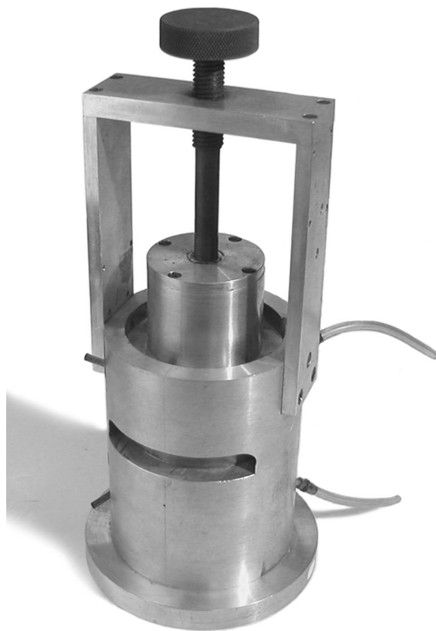
Fig. 9. Very early four pi gas flow proportional counter from Hanford (ca. 1950).
