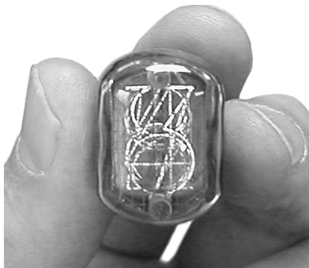
Fig. 13. Nixie tube (1960's). Which numbers can you make out?
