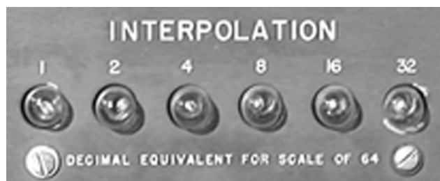
Fig. 11. Display for a scale of 64 binary scaler (late 1940's).
