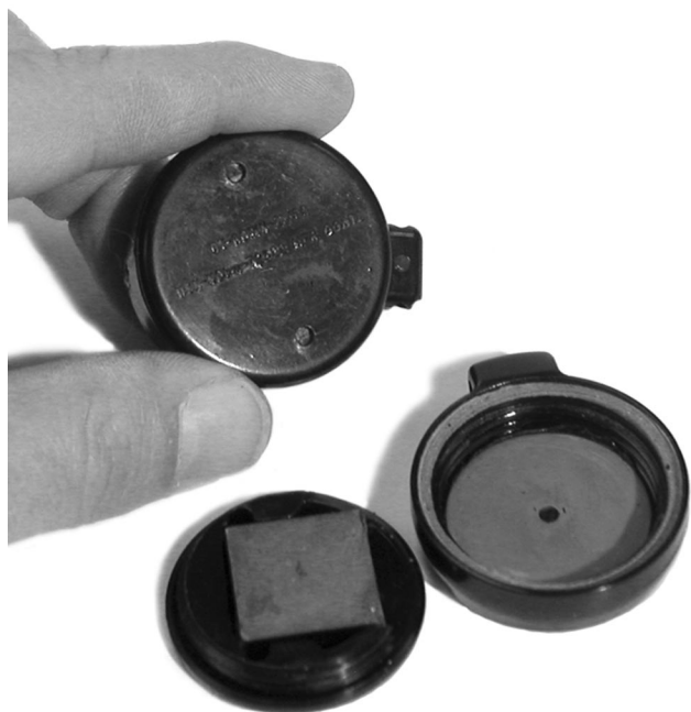
Fig. 17. Two DT60 radiophotoluminescent glass dosimeters used by the U.S. Navy (ca. 1960). The lower of the two has been opened so that the square block of RPL glass can be seen.
