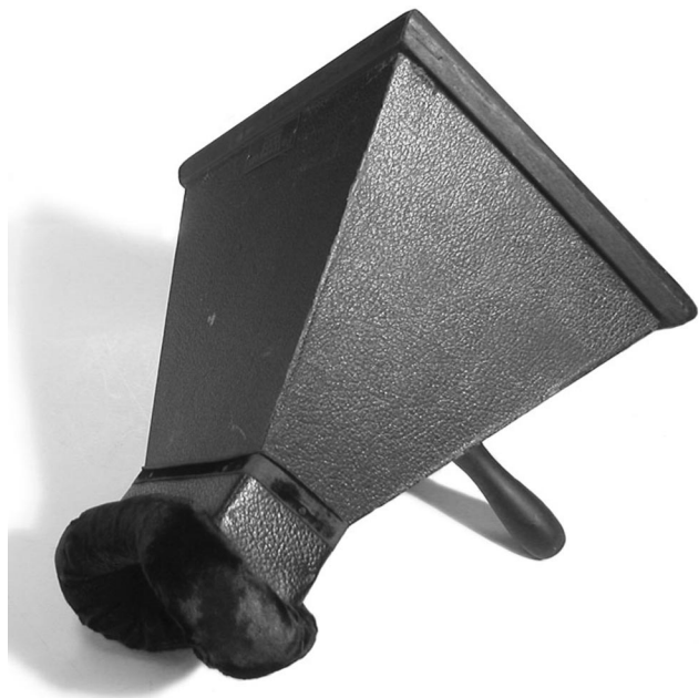
Fig. 14. Hand-held fluoroscope manufactured by the Patterson Screen Company (ca. 1920's).
