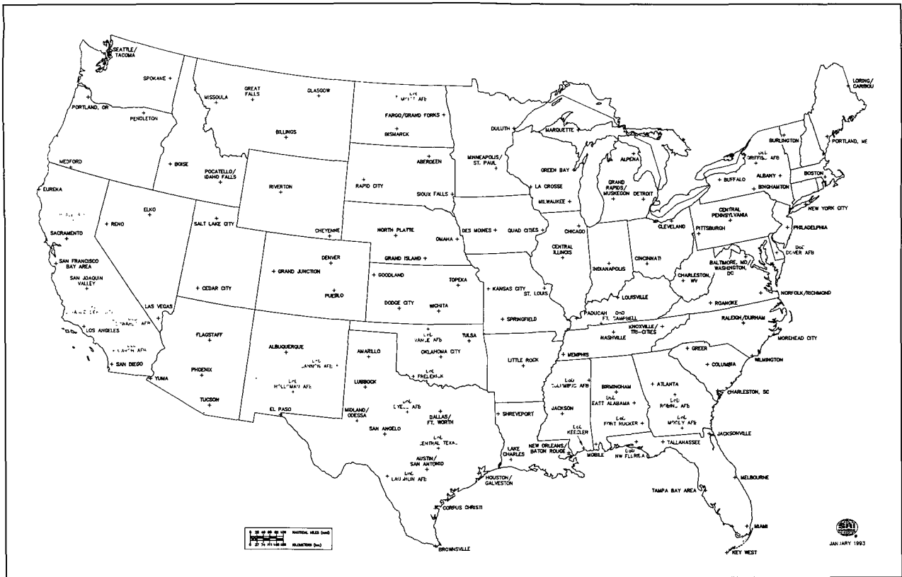
FIG. 2. Location of WSR-88D Radar Data Acquisition (RDA) units in the contiguous United States when installation is completed in 1996. A site will be added in the Fort Polk, Louisiana, area.
