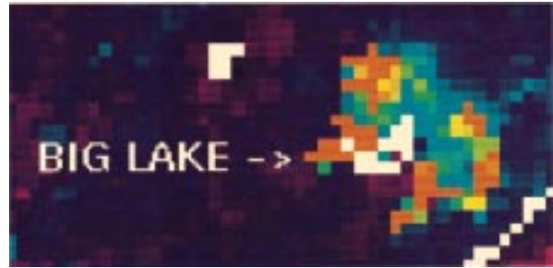
FIG. 11. NOAA AVHRR 3.7- \mu\text{m} image, 1349 LST 5 June 1996, showing fire-affected pixels using a false color table (red = hot, blue = cold).
