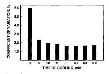
FIGURE 2. Precision of Absorbance Measurements after Various Cooling Times.
