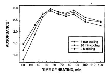
FIGURE 1. Effects of Time of Heating (at 87°C) and Time of Cooling (at 23°C) on Absorbance of Reaction Product.
