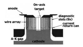
FIG. 3. Cross-section view of the Z diode with on-axis annular target. There are nine cutaway slots in the current-return can for diagnostic access. The Z machine is configured with the anode physically on the top of the target; other machines, such as Saturn, are configured with the anode down. The power from the magnetically insulating transmission lines flows to the diode through the gap in the lower part of the figure.
