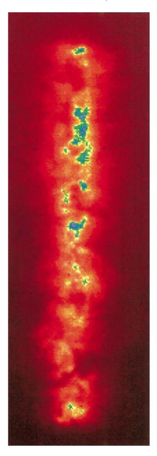
FIG. 20. View of 200–280-eV pinch radiation taken from  $88^{\circ}$  at Z (from Deeney, Douglas, et al., 1998, reprinted with kind permission of C. Deeney). The radiation is created by the stagnation of a nested wire array on-axis. The diameter of the radiating zone is approximately 2 mm. The initial diameter of the outer (inner) wire array was 40 mm (20 mm). The current waveform was similar to that shown in Fig. 4 [Color].
