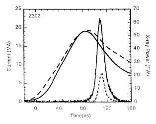
FIG. 29. The measured currents and x-ray powers from shot Z302, a 40-mm-diameter, 96-wire array with 20.3- $\mu$ m-diameter titanium wires. The load (solid) and MITL (dashed) currents are shown, along with the total power (solid) and kiloelectron-volt (dashed) x-ray powers (from Deeney *et al.*, 1999a, reprinted with kind permission of C. Deeney).
