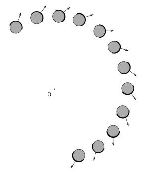
FIG. 24. Left-right asymmetric coating. Shown in heavier lines are the areas coated by material with a lower sublimation energy, which will ablate early in the pulse. The direction of the ablation flow is shown by arrows. Diameters of the wires are grossly exaggerated. Only part of the array is shown. Current flows into the paper.
