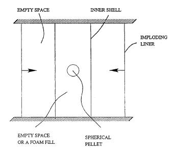
FIG. 33. Schematic of a dynamic hohlraum experiment.
