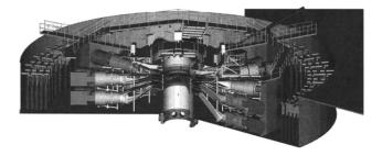
FIG. 2. Schematic of the Z facility. The diameter of the facility is 30 m. The outermost part is formed by Marx generators. They are connected to 36 water-insulated transmission lines which, in turn, feed magnetically insulated vacuum transmission lines converging at the diode. The diode is situated inside the central tank.
