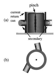
FIG. 31. Sideview (above) and end-on view (below) of a configuration with secondary hohlraums attached to the main one; this eliminates the effect of a direct irradiation of the sample by the pinch plasma.
