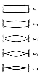
FIG. 6. Producing a quasispherical implosion with an initially cylindrical liner of varying thickness. The liner is thicker near the equatorial plane (see Drake *et al.*, 1996).
