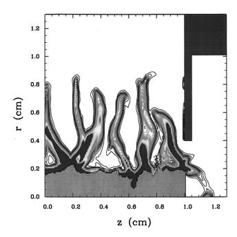
FIG. 22. Numerical results showing the possibility of current disruption by the m=0 mode (a 40-mm-diameter tungsten wire array on PBFA-Z after impacting a 2.5-mm-radius foam). From Peterson *et al.*, 1999, reprinted with kind permission of D. Peterson.
