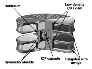
FIG. 35. A static hohlraum with two *Z*-pinch radiation sources situated at the ends.
