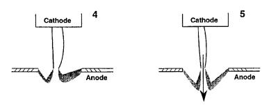
FIG. 8. Possible scenario of the implosion of a wire array in the case of a hollow anode. The picture is made deliberately asymmetric to emphasize the statistical character of the bridge formation.
