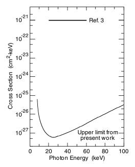
FIG. 4. Upper limit of the cross section for photon-induced deexcitation of the 31-yr <sup>178</sup>Hf isomer through the 4-s, 8<sup>-</sup> isomer from the measurements reported here. The value for this cross section reported in Ref. [3] is also shown. Other values reported by this group in the references cited in Ref. [6] range from  $2 \times 10^{-22}$  to  $2 \times 10^{-21}$  cm<sup>2</sup> keV. The present limits are substantially below all previously reported values.
