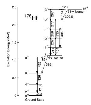
FIG. 1. Energy level diagram showing the decay of the 31-yr <sup>178</sup>Hf isomer. The transition energies are labeled in keV. Those transitions that were reported to be enhanced in [3,6] are highlighted.
