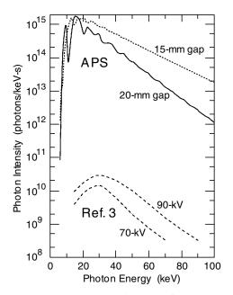
FIG. 2. The calculated photon intensity from the Advanced Photon Source, incident on the 2-mm-diameter area of the target material in the present experiment, for the two tapered settings of the undulator gap that were used. The photon intensities given in Refs. [3,6] for the 70- and 90-kV setting of the dental x-ray machine on a 1-cm diameter target are also shown.
