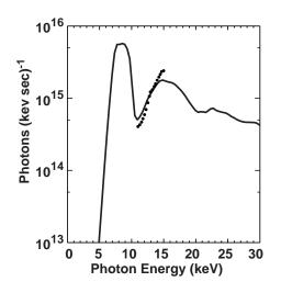
FIG. 2. Comparison of the calculated (line) and measured (dots) photon intensity from the advanced photon source incident on the  $HfO_2$  target.
