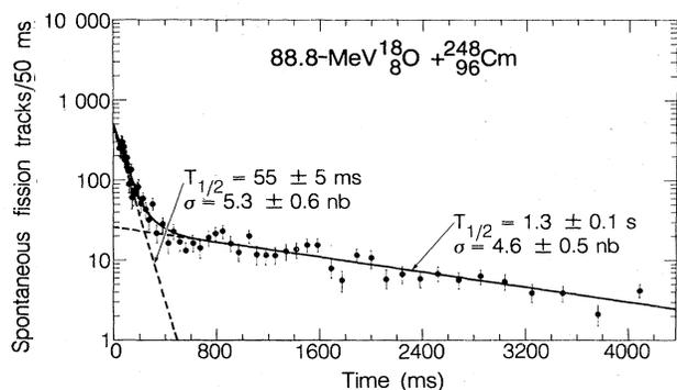
FIG. 6. Decay curve for the SF events observed in the reaction 88.8-MeV  $^{18}\text{O} + ^{248}\text{Cm}$ . The dashed lines show the amounts of the 55-ms and 1.3-s components computed in the fit; the solid curve is the sum of these components. The 55-ms component is probably due to  $^{262}\text{Rf}$ . The 1.3-s component has not yet been identified but is briefly discussed in Sec. III K 3.
