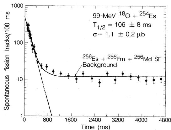
FIG. 7. Decay curve for the reaction 99-MeV  $^{18}\text{O} + ^{254}\text{Es}$  indicating that a 106-ms SF activity is produced. The dashed line shows the amount of the 106-ms component computed in the fit; the solid curve is the sum of this component and SF background. Although this  $\sim 100$ -ms activity could not be assigned, the production cross section is very large compared to our other SF activities.
