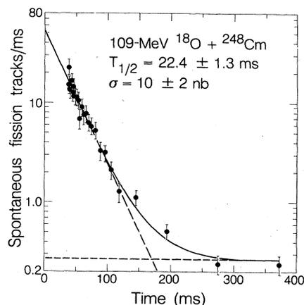
FIG. 4. Decay curve for the reaction 109-MeV  $^{18}\text{O} + ^{248}\text{Cm}$  showing a 22-ms SF activity. This half-life is indistinguishable from the half-lives deduced from the data in Figs. 3(a)–(c). The dashed lines show the amounts of the  $^{256}\text{Fm}$  background and the short-lived component determined in the fit; the solid curve shows the sum of these components.
