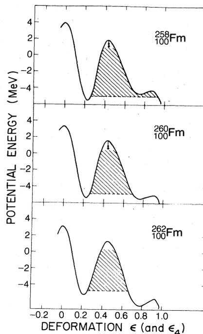
FIG. 9. Calculated fission barrier potentials plotted against the deformation parameter  $\epsilon$  for heavy isotopes of fermium (Ref. 6). Beyond  $^{258}\text{Fm}$  the second peak and second minimum are below the ground state energies shown as the horizontal dashed lines at the bases of the cross-hatched areas. This leads to a drastic decrease in the SF half-lives.
