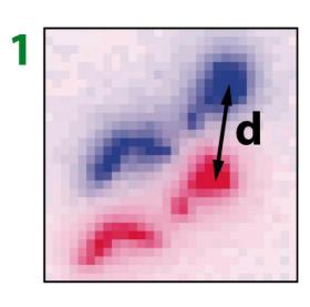
The stereo disparity **d** is unambiguously related to the water surface distance
