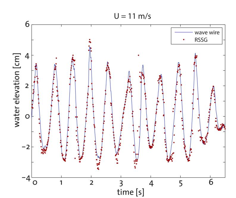
Comparison of capacitance type wave wire (blue line) and surface elevation from stereo with the RSSG (red dots). Data from experiment at Marseille wind-wave facility.
